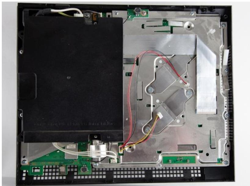
7. Connect the 3K3y 60 way FFC to the PS3 BD drive, fold it around the PS3 BD drive
