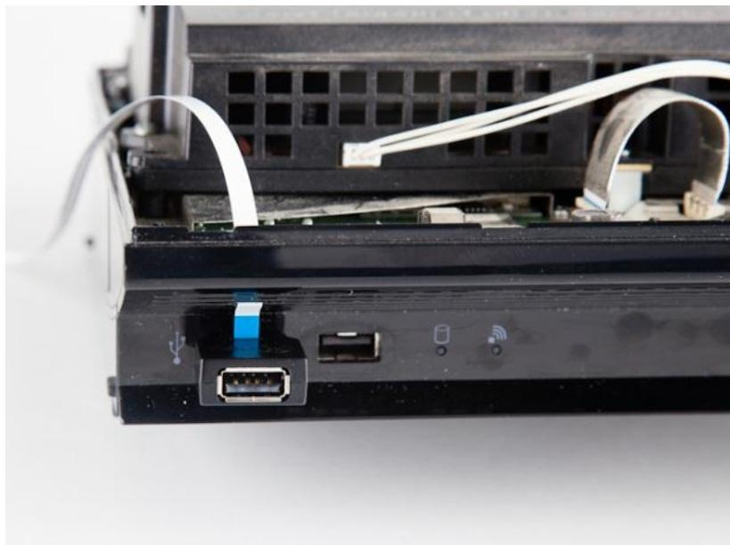
18. Connect the 3K3y 4 way FFC to the 3K3y PCB ZIF connector marked USB. The 4 way FFC should be routed tidily and may be secured with tape. Note, the blue plastic reinforcement of the 4 way FFC must be facing up.
