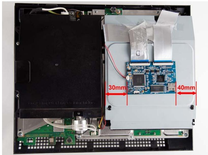
14. With a sharp knife or wire cutters remove part of the plastic case as shown
