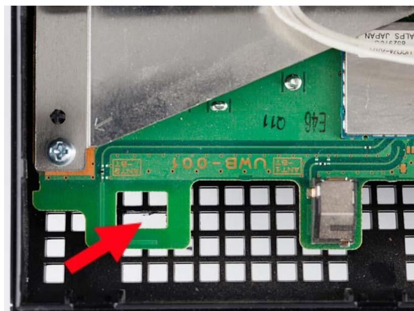
15. Pass the 3K3y 4 way FFC through the hole made in step 14, take care not to damage the FFC
