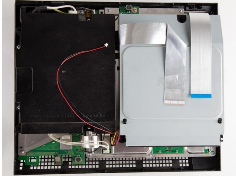
10. Place the 3K3y PCB as shown below, secure the PCB using the supplied double sided sticker.
