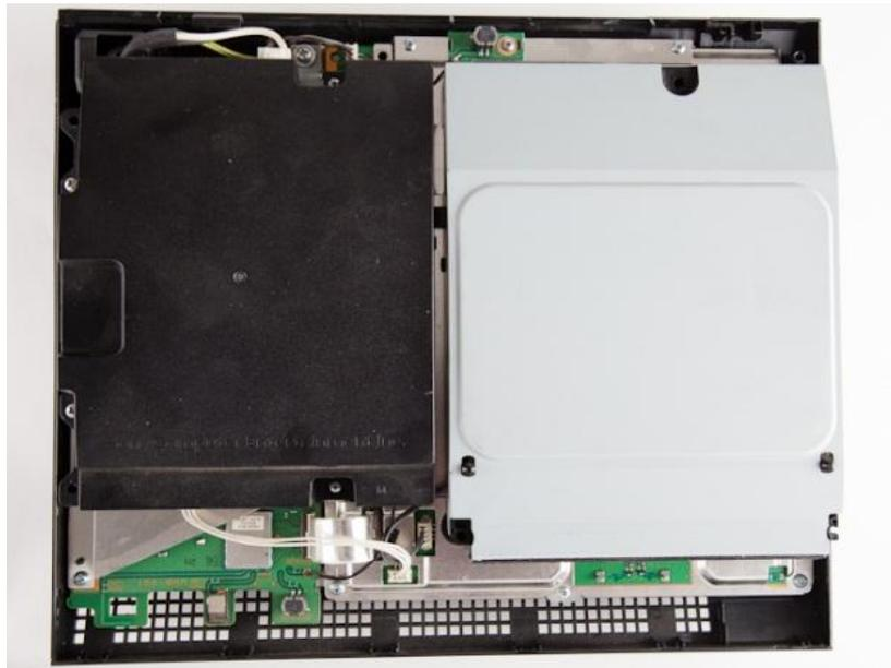
4. Disconnect the PS3 BD drive power cable from the PS3 motherboard
