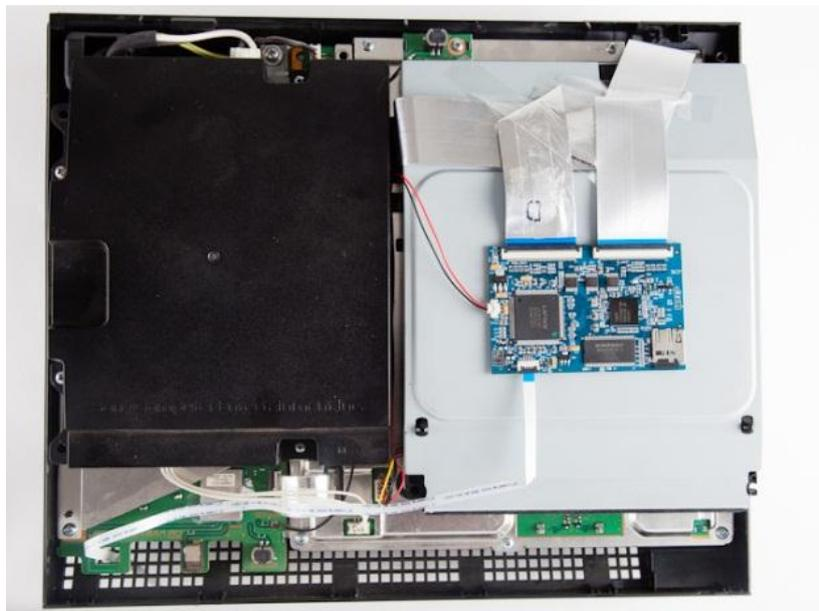
20. Carefully replace the top cover of the PS3, ensure that it does not interfere with the 3k3y PCB. Replace the top cover retaining screws.
