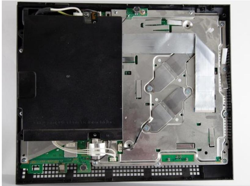
6. Connect the 3K3y power Y lead to the PS3 motherboard, ensure the double end of the Y lead is connected to the PS motherboard
