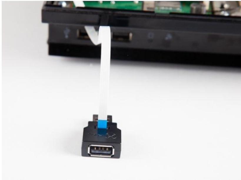
17. Plug the USB adapter into one of the PS3's USB sockets
