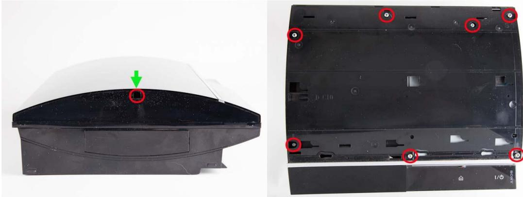
3. Remove the retaining screws and top cover from your PS3
